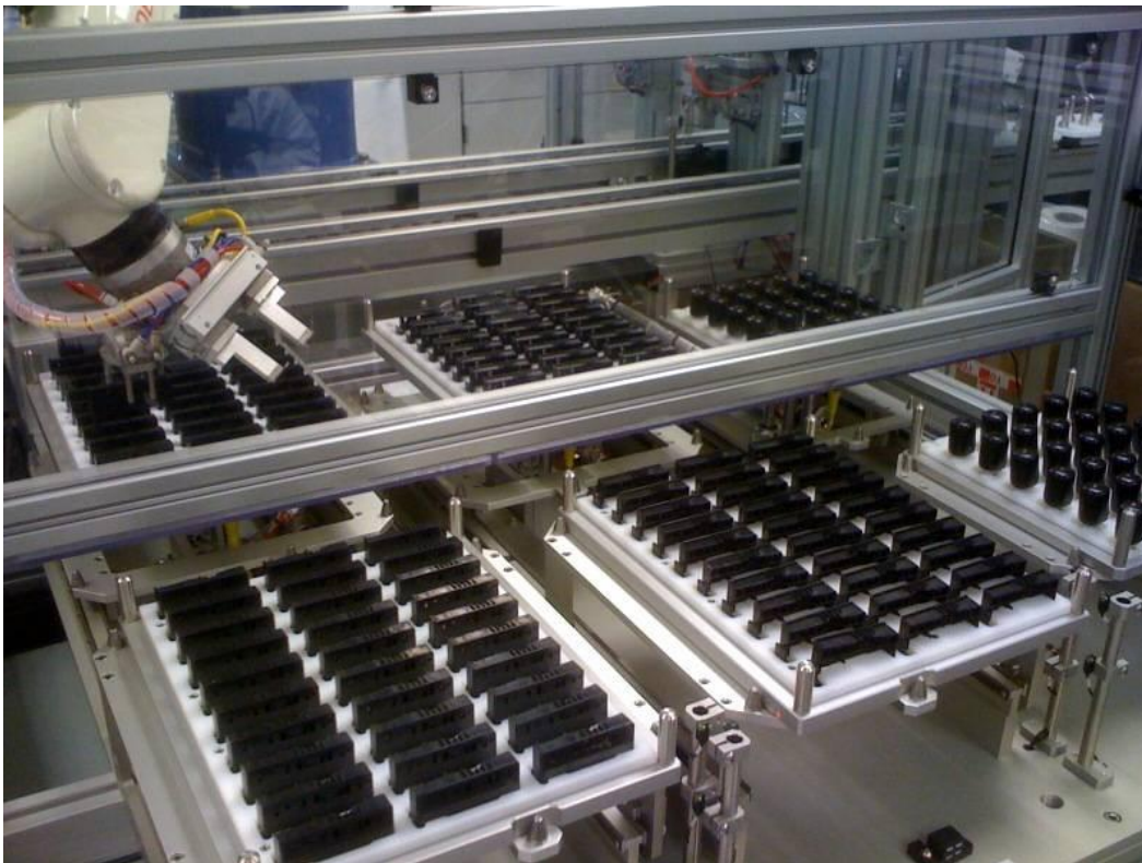
Tray Station Shown From Operator Loading Position (Doors Open)
