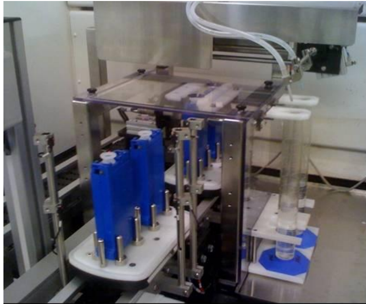
Pallet Shown Entering Fill Station with Two Empty Reservoirs Loaded
